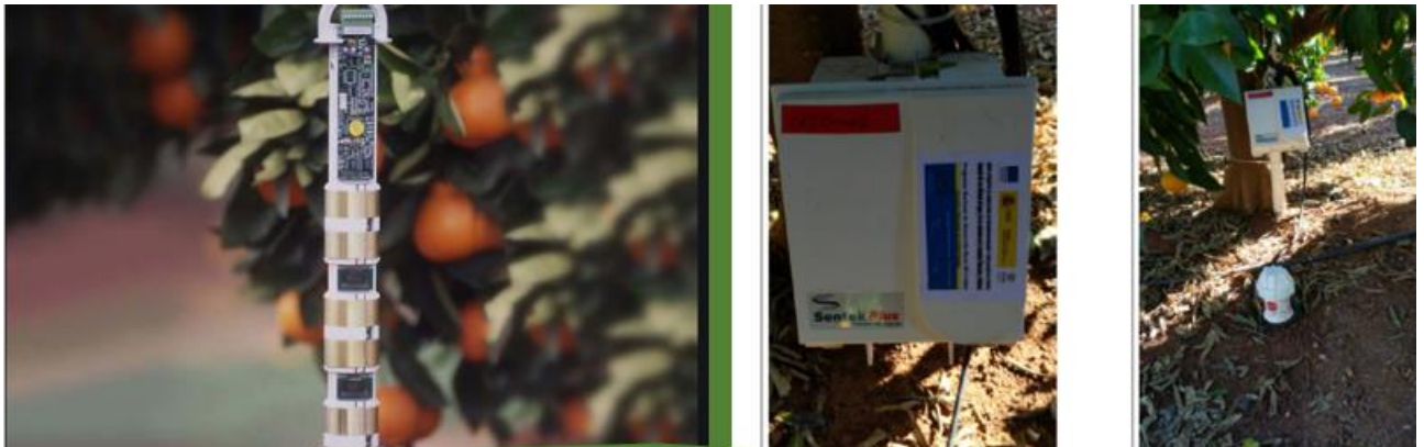
Figure 4: Capacitance probes, type Enviroscan Sentek, 3 levels of sensing at 20, 50 and 75 cm.
